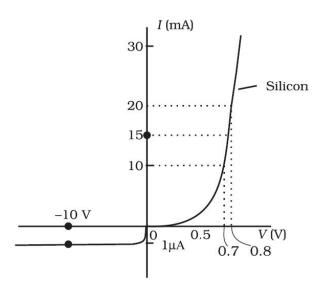
The V-I characteristic of a diode is shown in the figure. The ratio of the resistance of the diode at I = 15 mA to the resistance at V = -10 V is
